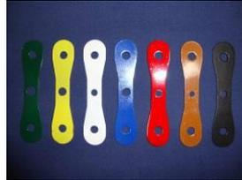
**Weak links must also be inspected before hook-up to the Glider at each launch for damage and correct load rating**
