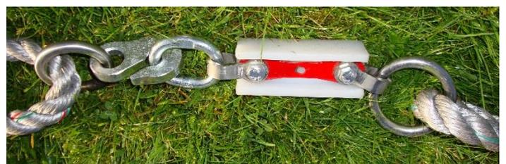
It is also recommended for safety that only one weak link holder assembly is connected, rather than the practice of having 2 or 3 attached all the time.
