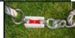
Weak Link Assembly (Slot in housing towards Glider)
