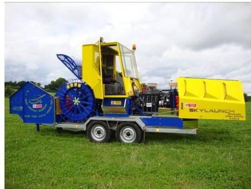
After over 30 years of experience using Big Block GM (Chevy) V8 engines for Glider launching they have proven to be the most suitable engines for these high load / short duration applications and there is no other engine which will give these characteristics for as low a price to buy, operate or repair.
